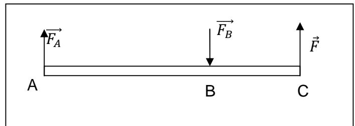
$$F_B = \frac{L}{a} F \quad \text{et} \quad F_A = \left( \frac{L}{a} - 1 \right) F = \frac{(L-a)}{a} F$$
