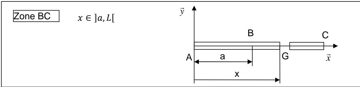
$$\{\tau_{coh}\}_G = + \left\{ \begin{matrix} F\vec{y} \\ \vec{0} \end{matrix} \right\}_G = \left\{ \frac{F\vec{y}}{\overrightarrow{GC} \wedge (F\vec{y})} \right\}_G = \left\{ F \begin{matrix} \vec{y} \\ (L-x)\vec{z} \end{matrix} \right\}_G = \left\{ \begin{matrix} N = \mathbf{0} \\ T_y = F \\ T_z = 0 \end{matrix} \quad \begin{matrix} M_t = \mathbf{0} \\ M_{fy} = \mathbf{0} \\ M_{fz} = F(L-x) \end{matrix} \right\}_G$$
