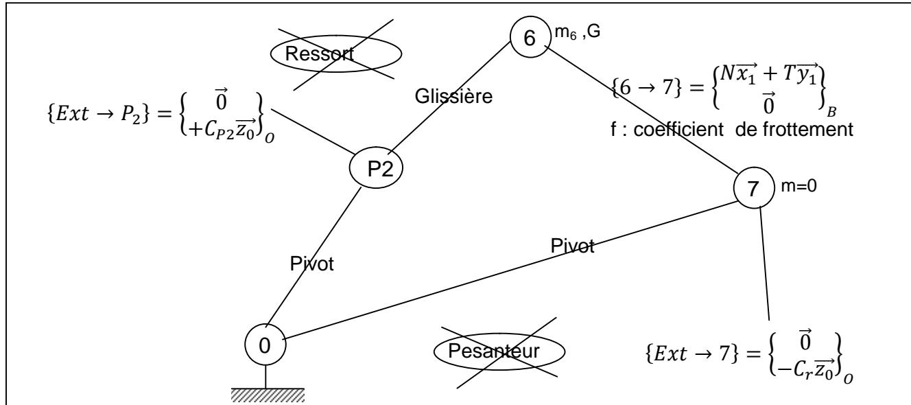
11°- PFD appliqué à (6) :  $\{P_2 \rightarrow 6\} + \{7 \rightarrow 6\} = \left\{ \begin{array}{c} m_6 \overrightarrow{\gamma_{(G/R_0)}} \\ \vec{\delta}_G (6/R_0) \end{array} \right\}_G$
